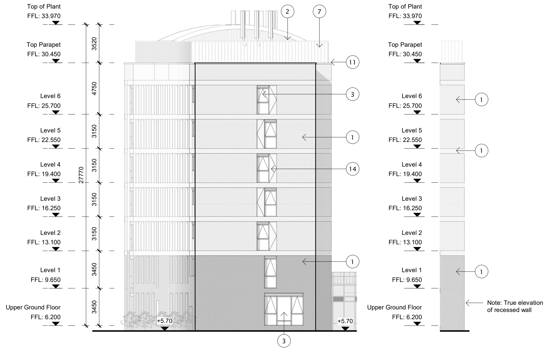
4 Block 2A - West Wing - South Elevations 1 : 200
